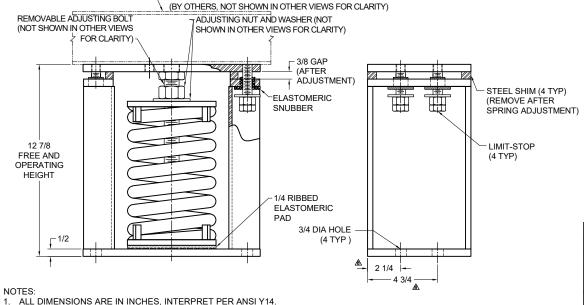
BOLT OR WELD EQUIPMENT SUPPORT BEAM TO MOUNT
